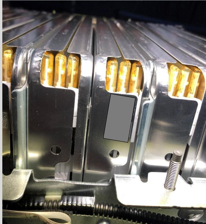
Detail of a battery module (constructed with a 4-cell configuration).
